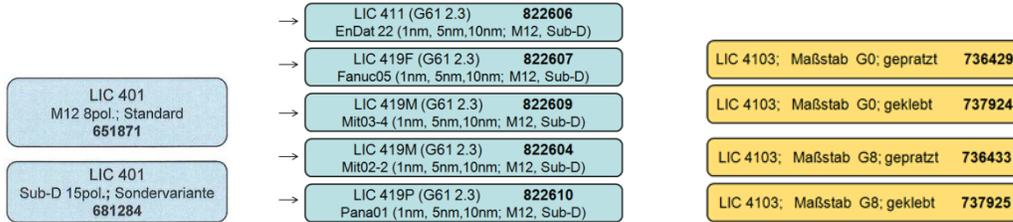
Starting with the introduction of the new **LIC 4100** series, the basic ID numbers for the **LIC 411** and **LIC 419 scanning heads** will only be assigned for the respective interface. Other variants, such as resolution, accuracy grade, connector type, will be listed as variants.
